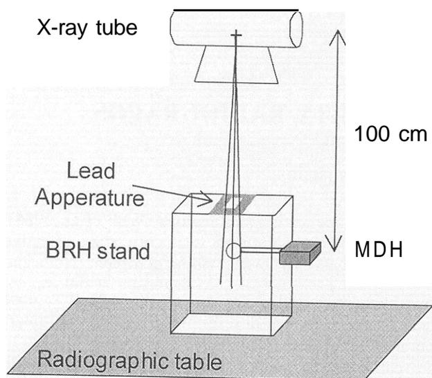
Fig. 1. Experimental setup of measuring tube output exposures.
