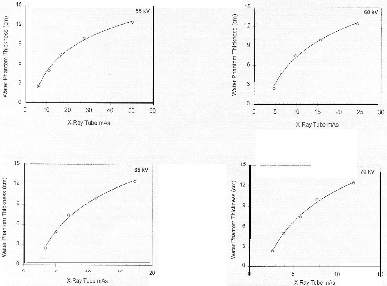
Fig. 4. Water phantom thickness required to generate a film with a gross film density of 1.4 vs. x-ray tube mAs (see text for details).
